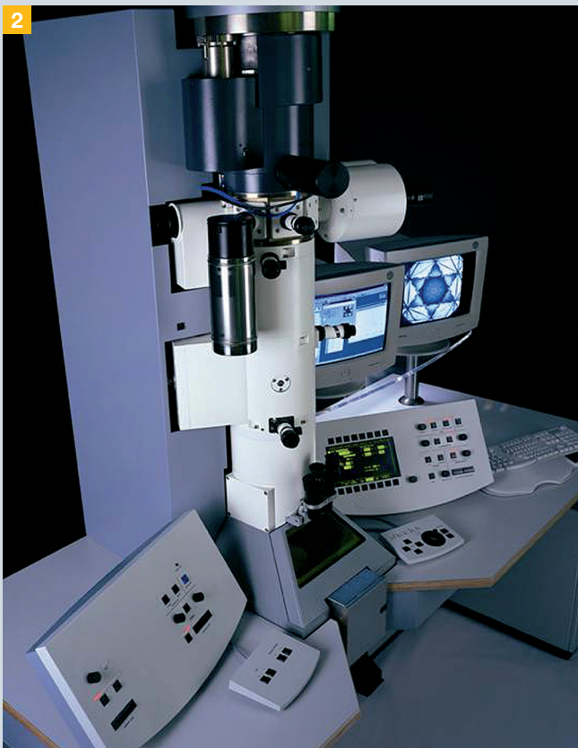
An energy-filtering transmission electron microscope. Elemental maps can be generated using its built-in energy filter in conjunction with digital image acquisition and image processing.
